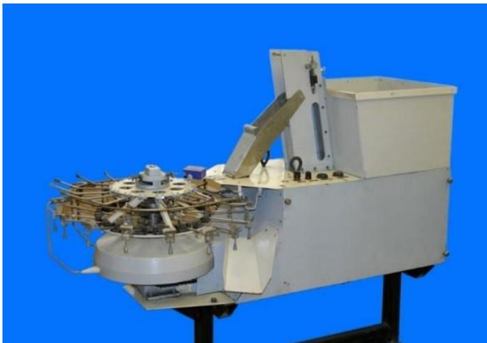
**Figure 5.** Upgraded automatic for dividing cocoons by the sex.
