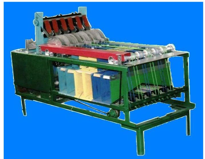
Figure 4. The cocoon calibration device
