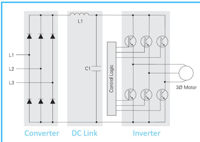
**Fig13: Circuit Diagram of inverter**
