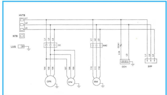
**Fig2: POWER CIRCUIT OF AIR CONDITIONER**
