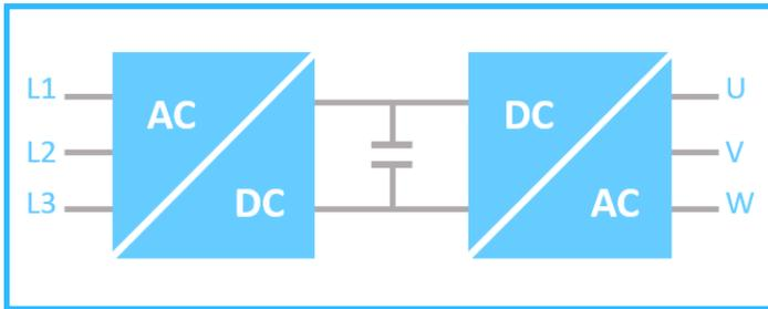
**Fig12: Block Diagram of inverter**
