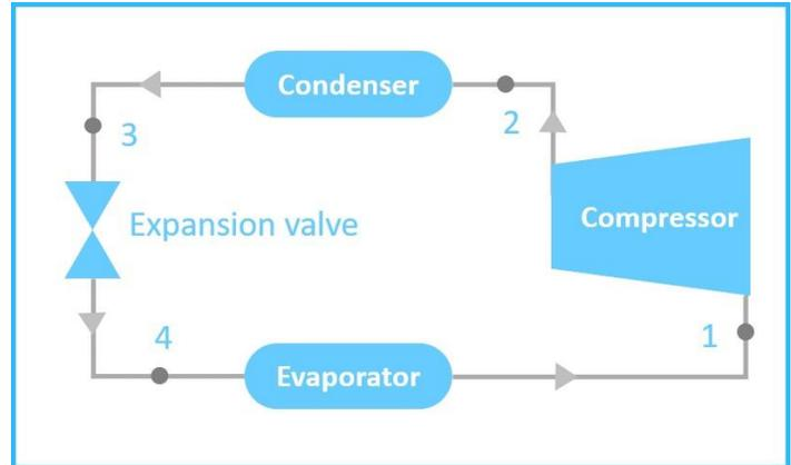
**Fig1: Refrigeration Circuit**
