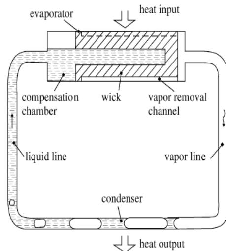
**Fig: A** schematic of the structure and principle of operation of a loop heat pipe
