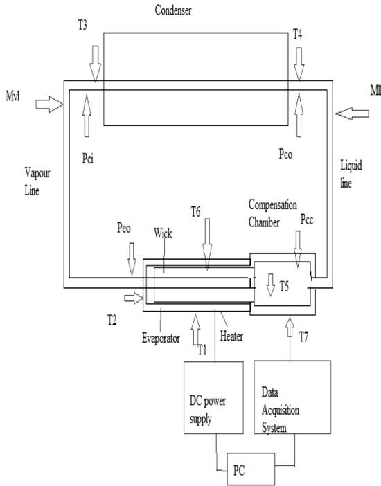
**Fig. Schematic of the Test Setup**
