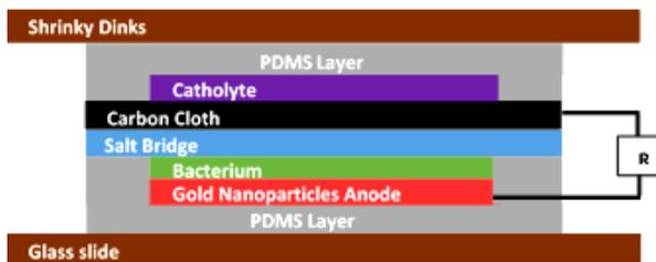
**Schematic 01:** Fabrication of Mini-MFC
