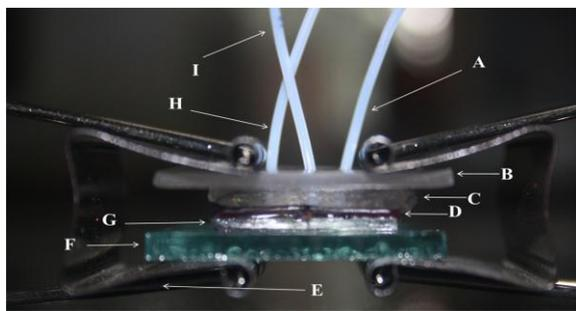
**Fig 01:** Lateral View of Mini-MFC Setup
