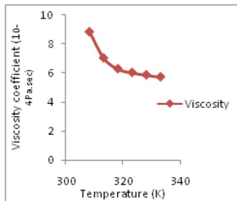
**Fig. 2** Variation of salt sugar solution (sss) viscosity with temperature
