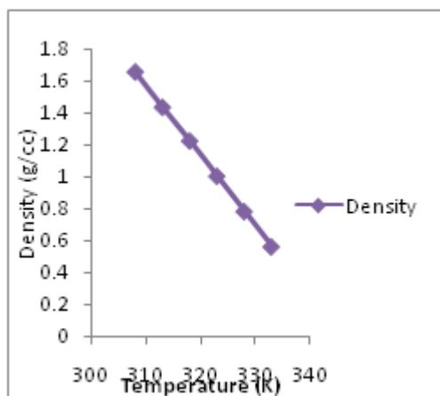
**Fig. 1** Variation of salt sugar solution (sss) density with temperature
