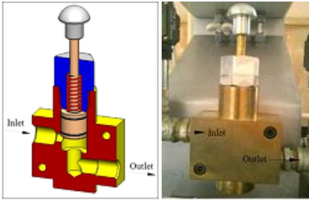
Figure 2. The Designed Hand Operated Safety Valve
