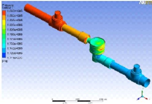
Figure 6. Pressure Distribution of Flow Volume
