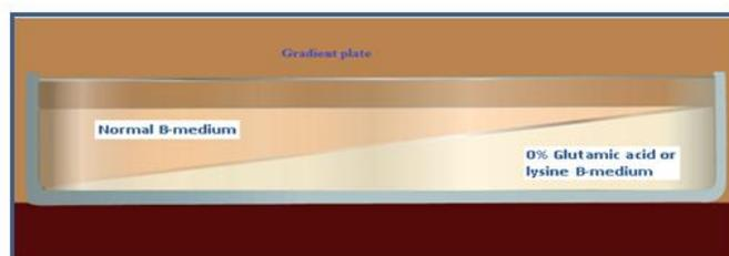
**Figure 3.** Gradient plate. A bottom layer (12.5 ml) of 0 % amino acid (glutamic acid or lysine or both) of B-medium agar and a top layer (12.5 ml) of normal B-medium agar. The amino acid in the top layer, diffuses into the bottom layer producing a gradient of chemical concentration from low to high and for that reason it is required that both layers must be in slant form until this gradient concentration is established across plate from 0 to 100 % of the intended amino acid.
