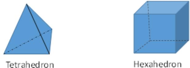
Figure 5 Element shape used in FEM
