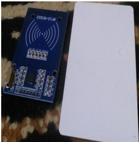
Figure 4. Pictorial view of the RFID sensor.
