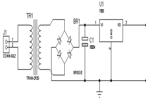
Figure 2. Circuit diagram of power supply
