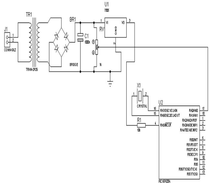
Figure 4. Circuit diagram of the power supply and the voltage sensor
