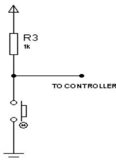
Figure 7. Circuit diagram of the trigger switch
