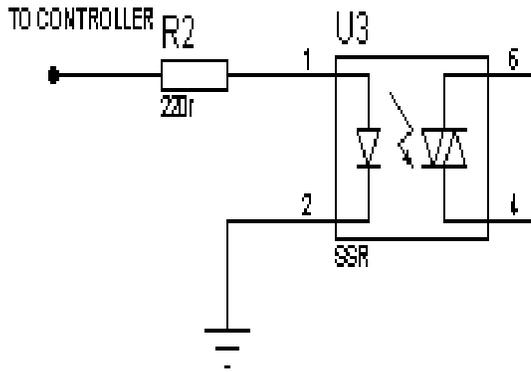
Figure 6. Circuit diagram the Solid State relay
