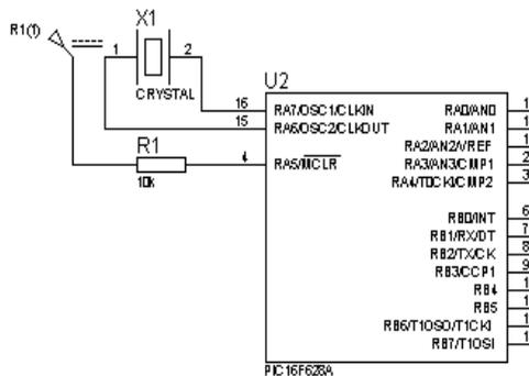
Figure 3. Circuit diagram of the controller
