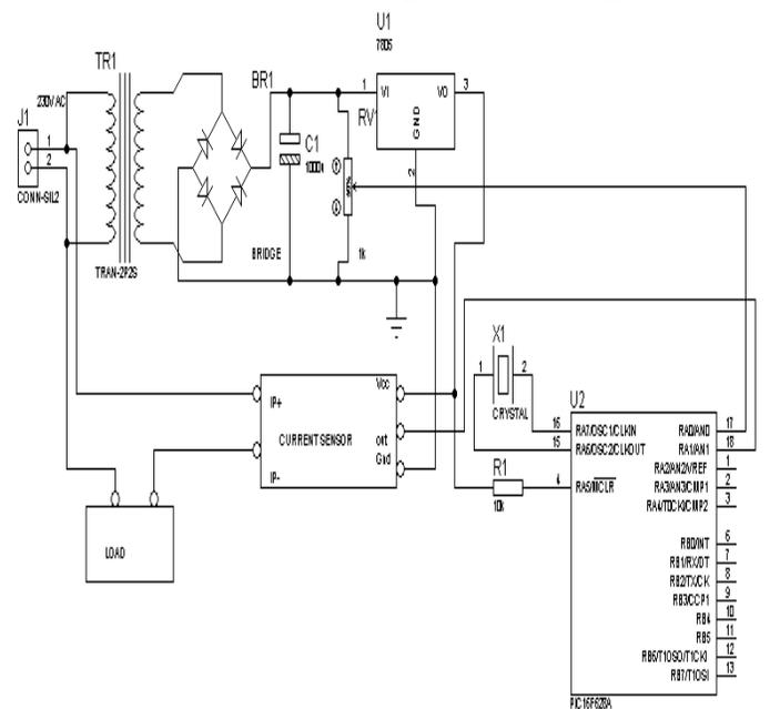
Figure 5. Circuit diagram of power supply, voltage sensor and current sensor connected to the controller
