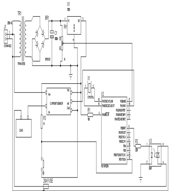
Figure 8. Complete circuit diagram of the system
