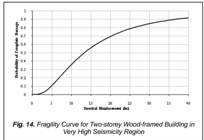
After this, the probability of complete damage is determined at each peak response. Therefore, the probabilities of complete damage are 0.0154 and 0.007 for one- and two-storey wood frame building in High seismicity region, and 0.1254 and 0.0722 for one- and two-storey wood frame building in Very High seismicity region. From the resulting values, the probability of collapse is determined by using the following equation.
