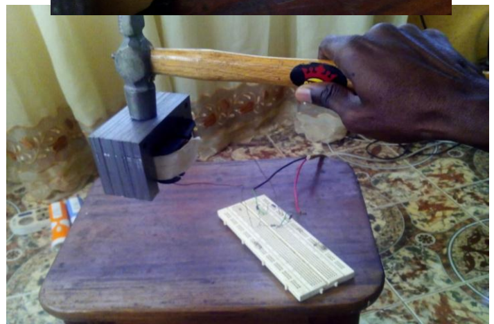
Figure 8: Pictures of the design of a rectified electromagnet (using a larger core). (The hammer was attracted to the magnetized core, as the hammer was pulled up and the core was attracted to it due to the strong magnetic field present).
