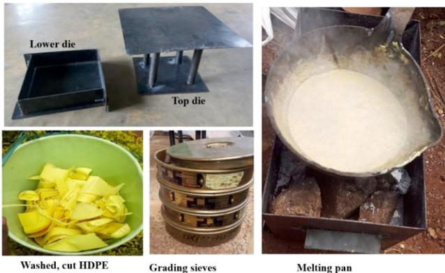
**Figure 1.** Materials and equipment used in the preparation of the composites
