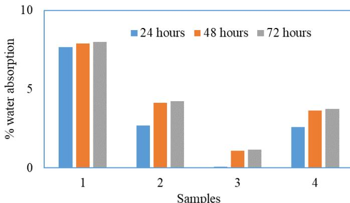
**Figure 3.** Percentage (%) water absorption for plastic-macadamia composites
