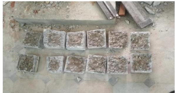
Fig: 4.5 chlorine penetration depth (after spraying 0.1M AgNO<sub>3</sub>)
