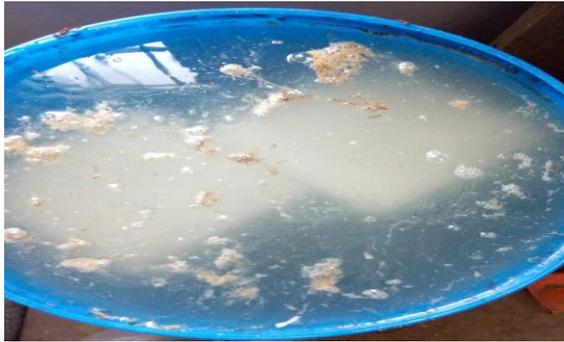
Fig 4.3 Cubes are under curing in acid solution
