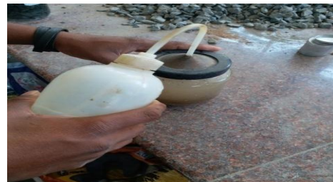
Fig.1 Specific Gravity of Natural river sand
