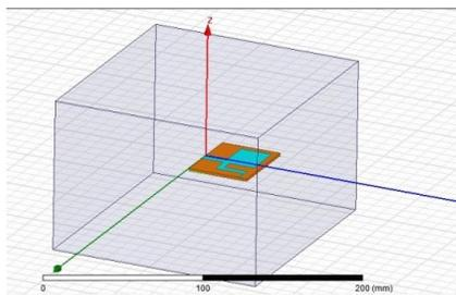
Figure 1: 3D view of Antenna implementation
