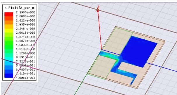
(b) H field of designed Antenna
