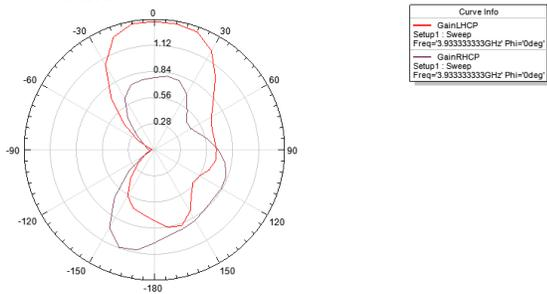
Figure 7(a): Measured Radiation Pattern at 3.933GHz
