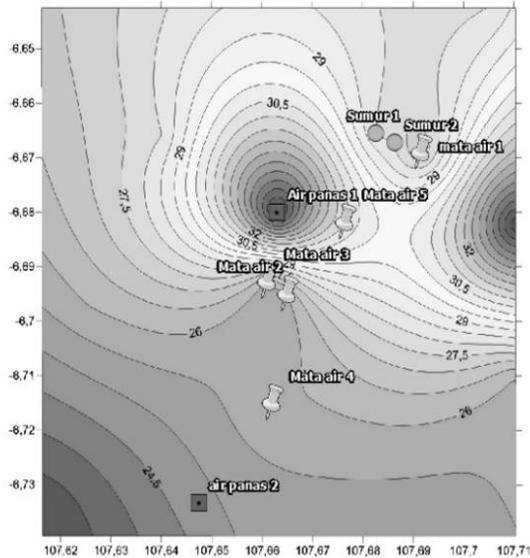
**Figure 5 Temperature measurement map**
