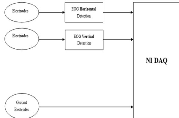
**Fig 2** Processing of EOG signal for drowsiness detection
