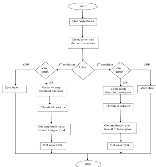
Fig 3 Flow diagram for determining peaks in LabVIEW
