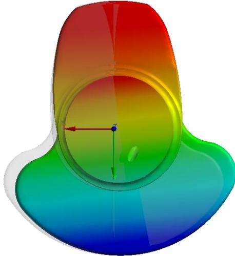
**Fig. 2** Deformation of the crank throw under unit torque
