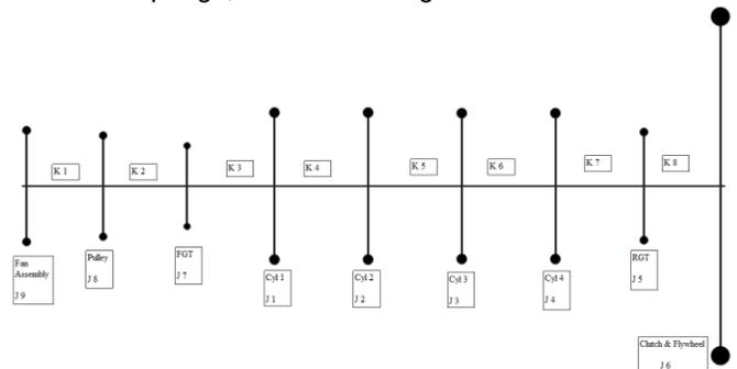
Fig. 1 Torsional spring-mass system
