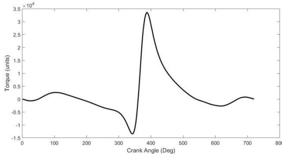
**Fig. 4** Typical Torque generated by a single cylinder
