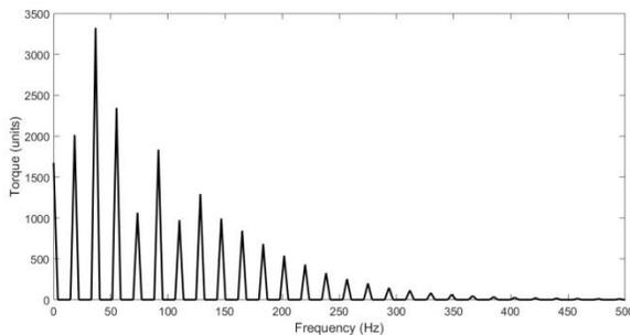
**Fig. 5** Frequency spectrum of the effective torque of a single cylinder
