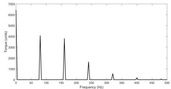
**Fig. 7** Frequency spectrum of the torque developed
