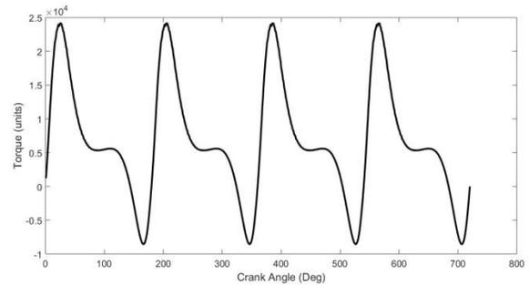
**Fig. 6** Effective torque developed by the engine
