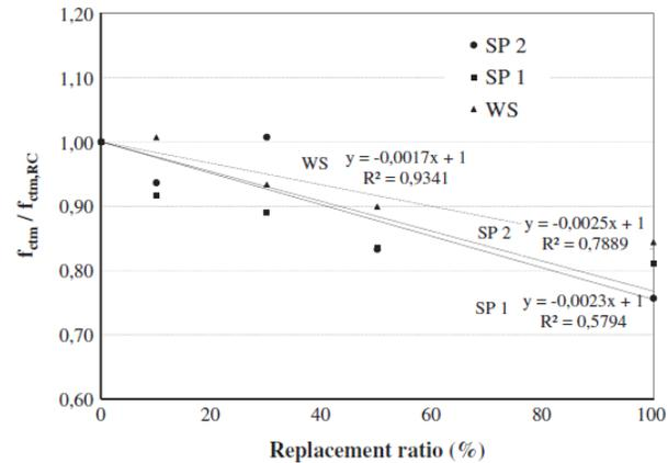
**FIG. 9.** FNA/FRCA replacement ratio and splitting tensile strength at 28-day of relative FRAC [19].
