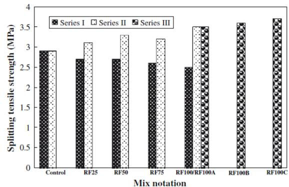
**FIG. 10.** RA-SCC Splitting tensile strength at 28 days in Series I, II, and III [10].
