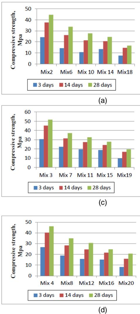
**FIG. 4** compressive strength of self-compacting concrete: a) SCC-control, b) SCC-fly ash, c) SCC-slag, d) SCC-fly ash & slag [13].
