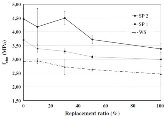
**FIGURE 8.** FNA/FRA replacement ratio and Splitting tensile strength at 28 days[19].
