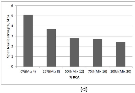
**FIG. 7.** Split tensile strength of SCC: a) SCC-control, b) SCC-fly ash, c) SCC-slag, d) SCC-fly ash & slag [13]
