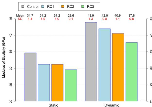
**FIG. 11.** dynamic and Static elastic modulus of different mixes [12].
