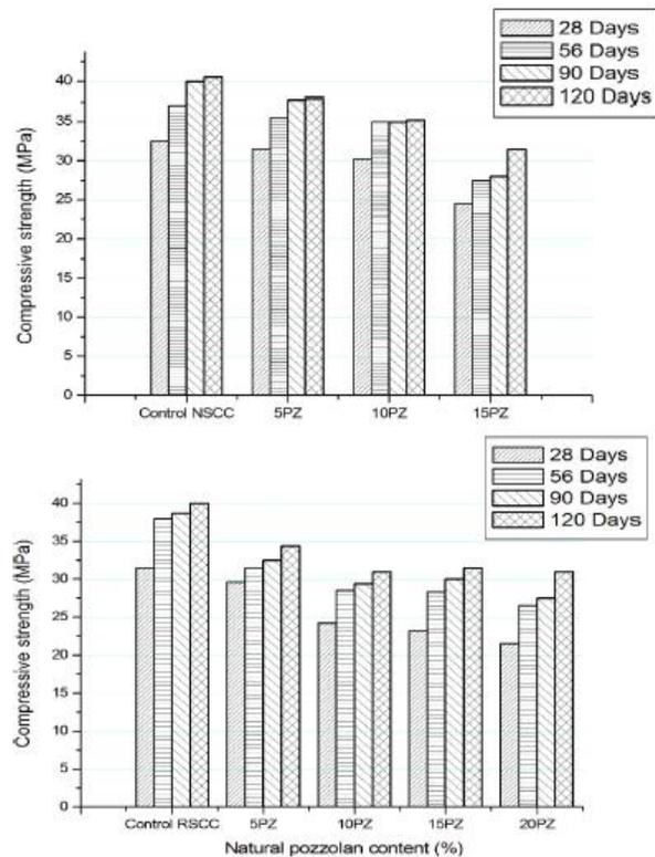
**FIG. 5.** RSCC and NSCC Compressive strength vs natural pozzolan content (%) [8].
