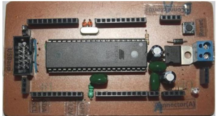
Figure 3. Main Board (ATmega32)
