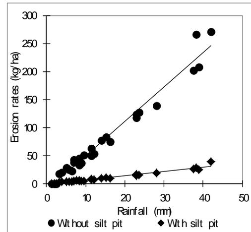
**Fig. 6.** Relationship of rainfall vs erosion rates occurred in the two experimental plots
