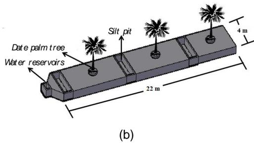
Fig. 3 The experimental plot setup (a) without silt pit (b) with silt pit
