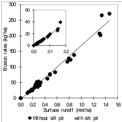
Fig. 7. Relationship between surface runoff vs erosion occurs in the two experimental plots
