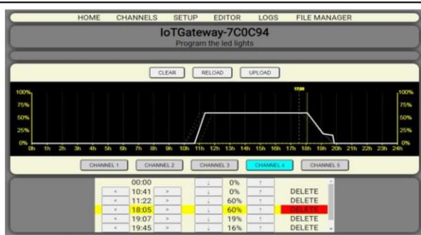
Fig. 15. An example user interface to program scheduler of an actuator by using mouse click event handler; the vertical axis shows the percentage of lights (using PWM); the horizontal shows the time with accuracy in a minute.
