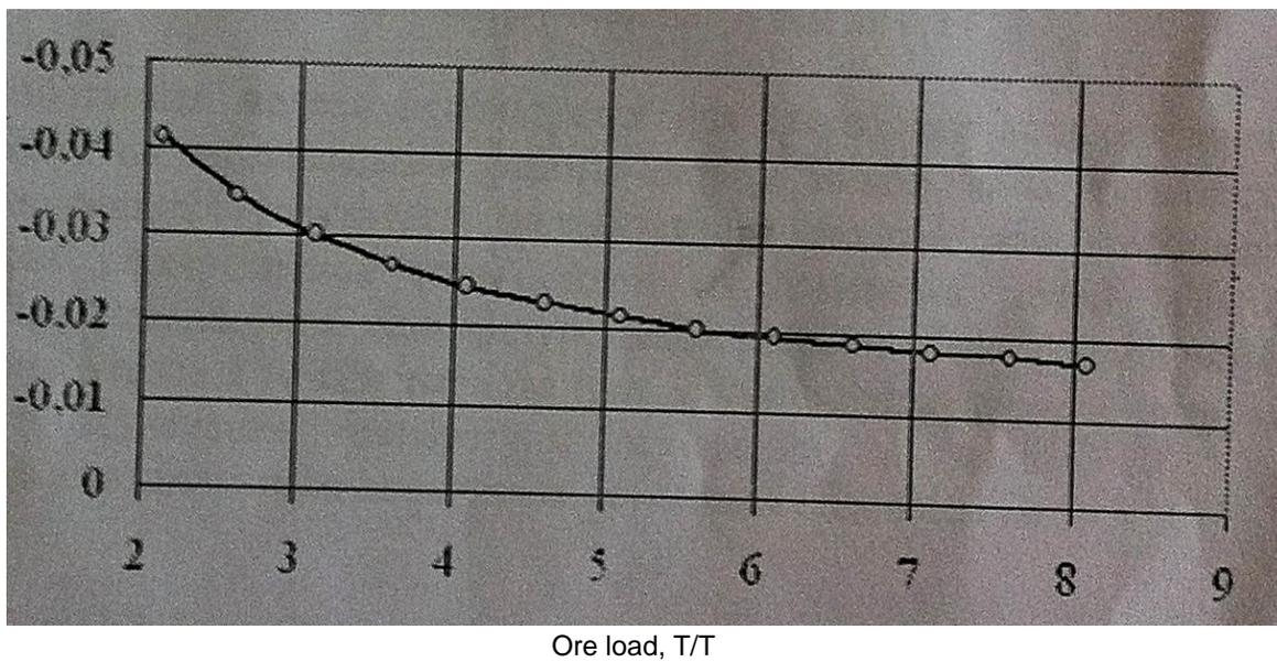
Fig. 1 Change in the level of indirect regeneration at the increase of ore load to 0.1
