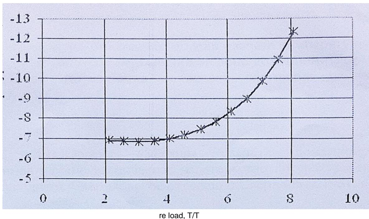
Fig 2 Change in temperature of peripheral gases when ore load is increased to 0.1
