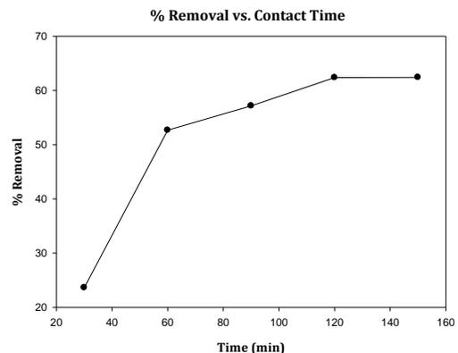
**Figure-2:** Effect of contact time on the removal of dyes by adsorption onto orange peel. (Initial concentration: 6g/mL, Amount of orange peel: 1.5 g and pH value: 7)
