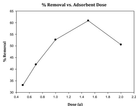
**Figure-1:** Effect of orange peels dose on the removal of dyes by adsorption onto orange peel. (Initial concentration: 6g/L. pH value: 7 and contact time: 90 minutes.)
