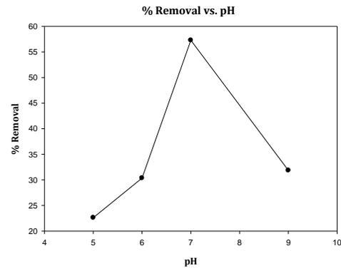
**Figure-3:** Effect of pH on the removal of dyes by adsorption onto orange peel. (Initial concentration: 6 g/L, amount of adsorbent: 1.5 g and contact time: 90 minutes.)
