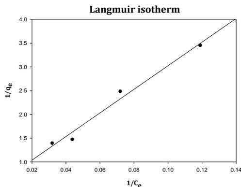
**Figure-4:** Langmuir isotherm for Deazol Black B EAN reactive dye onto orange peel (initial concentration: 20-60 mg/L; time: 180 minutes, pH: 6.5-7; room temperature).
