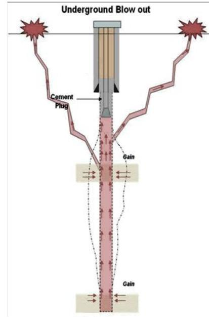
**Fig. 2. Underground blow out**
