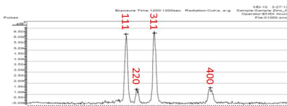
Figure 1: X-ray diffraction pattern of ZnSe thin film deposited on Zinc metallic substrate for 30secs under optimum experimental conditions.
