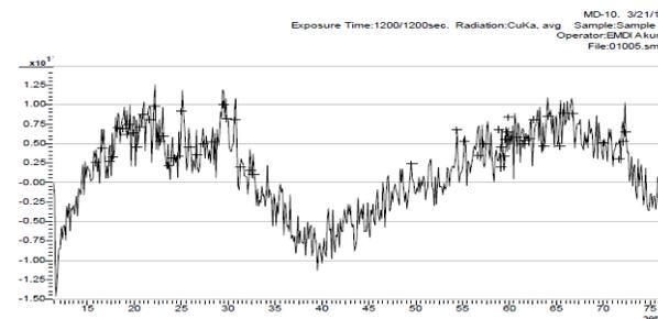
Figure 4: X-ray diffraction pattern of ZnSe thin film deposited on conducting glass (ITO) substrate for 30secs under optimum experimental conditions
