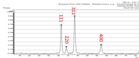
Figure 2: X-ray diffraction pattern of ZnSe thin film deposited on Zinc metallic substrate for 60secs under optimum experimental conditions.
