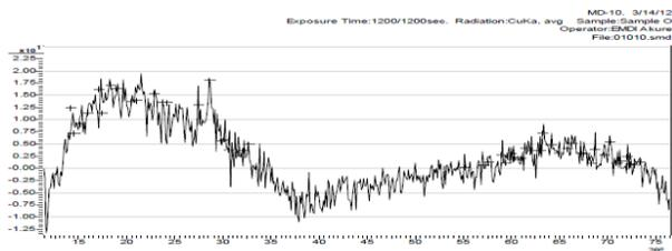
**Figure 5:** X-ray diffraction pattern of ZnSe thin film deposited on conducting glass (ITO) substrate for 60secs under optimum experimental conditions
