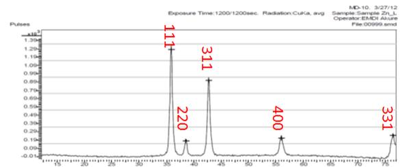
Figure 3: X-ray diffraction pattern of ZnSe thin film deposited on Zinc metallic substrate for 90secs under optimum experimental conditions.
