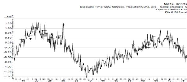
**Figure 6:** X-ray diffraction pattern of ZnSe thin film deposited on conducting glass (ITO) substrate for 90secs under optimum experimental conditions
