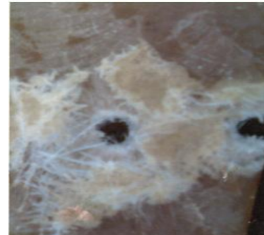
Fig. 6: Sample F, showing failure with complete perforation.
