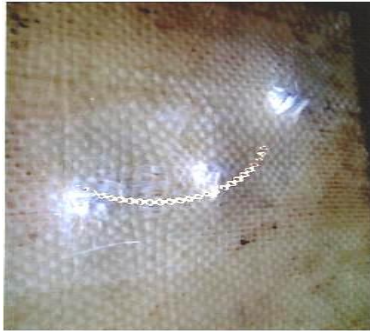
Fig 2: Sample D, showing minimal shattering by impact.
