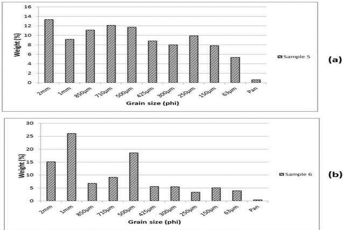
**Figure 3 (a) and (b) grain size distribution of samples 5 and 6**
