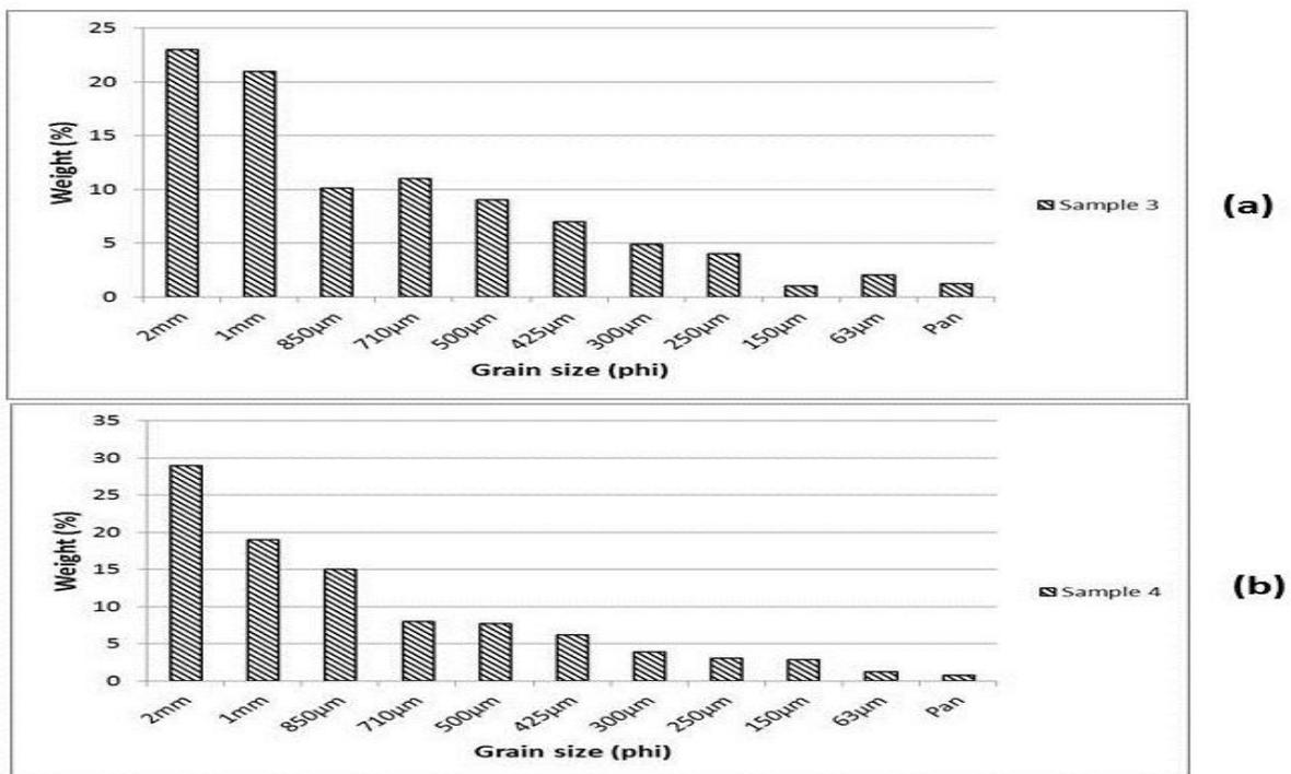
Figure 2 (a) and (b) grain size distribution of samples 3 and 4
