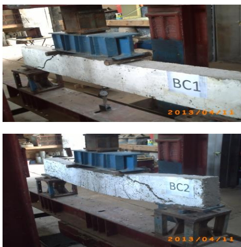
Fig.4 Failure pattern of Beams (CB1) and (CB2)
