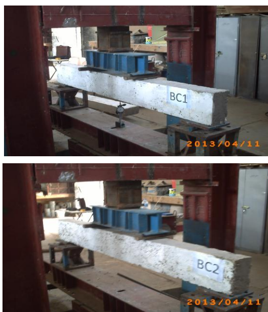
Fig.2 Test setup and instrumentation of beams
