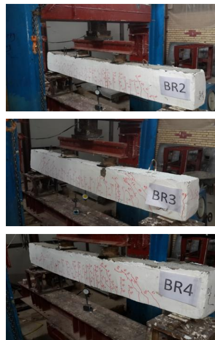
Fig.12 Failure pattern of strengthened and repaired beams
