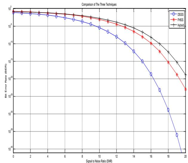
Fig.1 Comparison of SNR vs. BER for the three techniques
