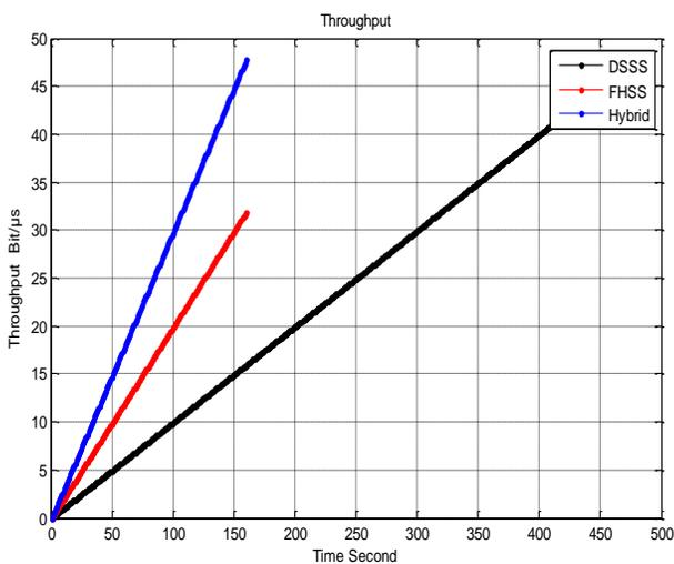
**Fig.3** Throughput comparison between DSSS, FHSS, and the Hybrid Technique
