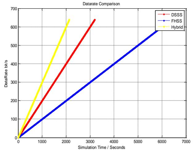
**Fig.4** Datarate comparison between DSSS, FHSS, and the Hybrid Technique
