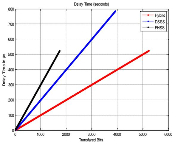
**Fig.2** Comparison of Delay time between DSSS, FHSS, and the Hybrid technique
