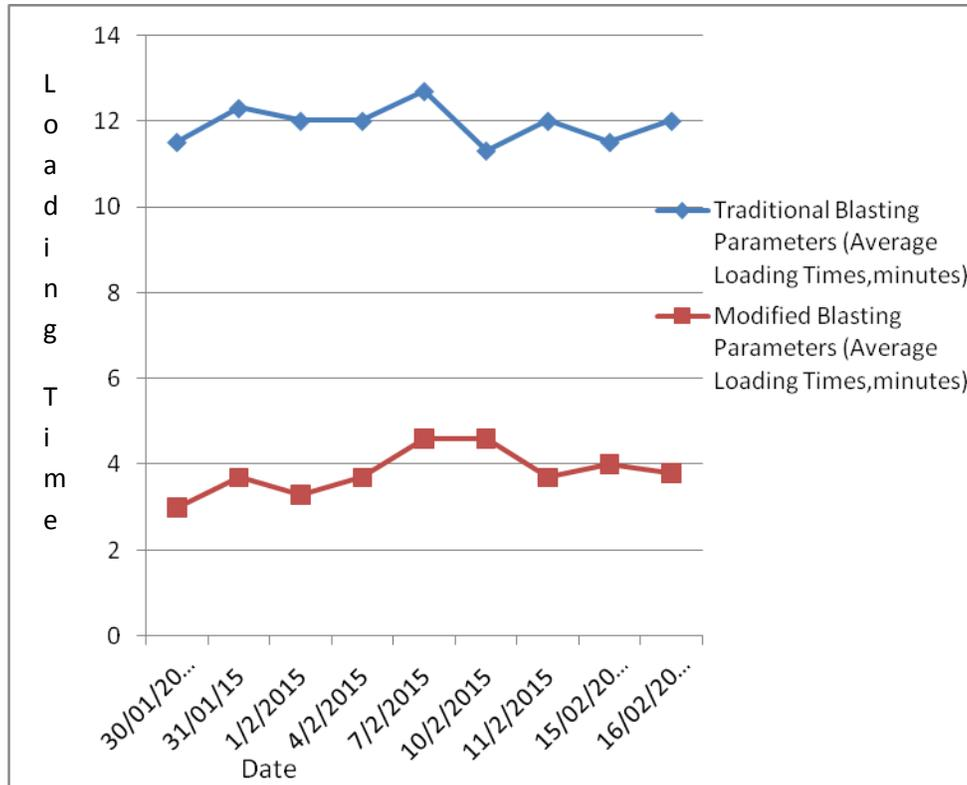
Figure 4: Shovel loading times for blasted material using both traditional and modified blast design parameters on different dates.
