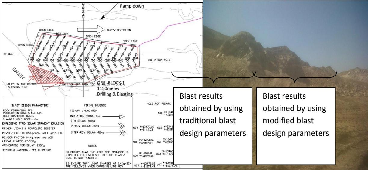
Figure 3: Drilling and blasting plan and blast results obtained by using both traditional and modified blasting design parameters.
