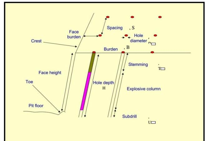
**Figure 1: Parameters considered in open pit bench blast design modified after (Anon, 2012)**
