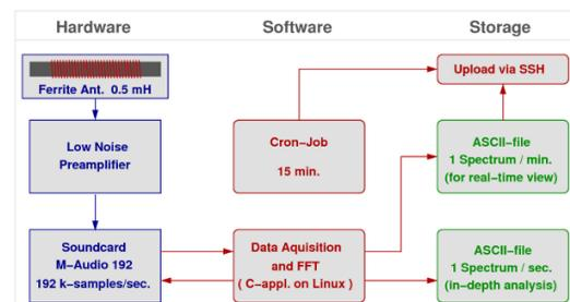
Fig 1: Block diagram of Kiel Longwave Monitor
