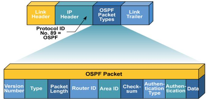
**Figure 2.1:** OSPF Message encapsulation. (Cisco Press “OSPF Message Encapsulation”, 1999)
