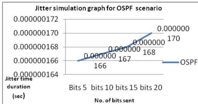
Figure 7: Jitter simulation graph for OSPF
