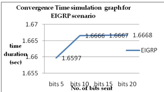
Figure4: Convergence time simulation graph for EIGRP protocol
