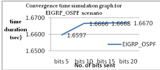
Figure 6: Convergence time simulation graph for EIGRP OSPF protocol.
