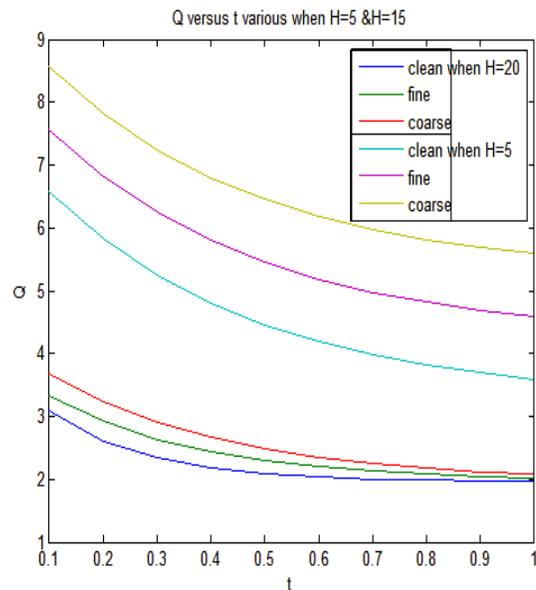
**Fig. 3** The effects of the magnetic field H on the flow rate 'Q' With time 't' for different values of H,  $\beta=0.2$ ,  $\gamma'=0.1$
