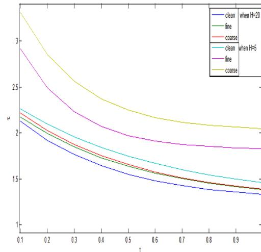
**Fig. 2** The Effects of the magnetic field H on the wall shear stress 'tau' With time 't' for different values of H,  $\beta=0.2$ ,  $\gamma'=0.1$
