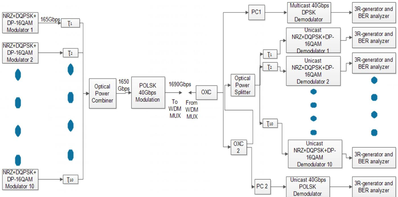
Fig.1. Schematic Design for transmission and reception of single unicast and multicast sub channels
