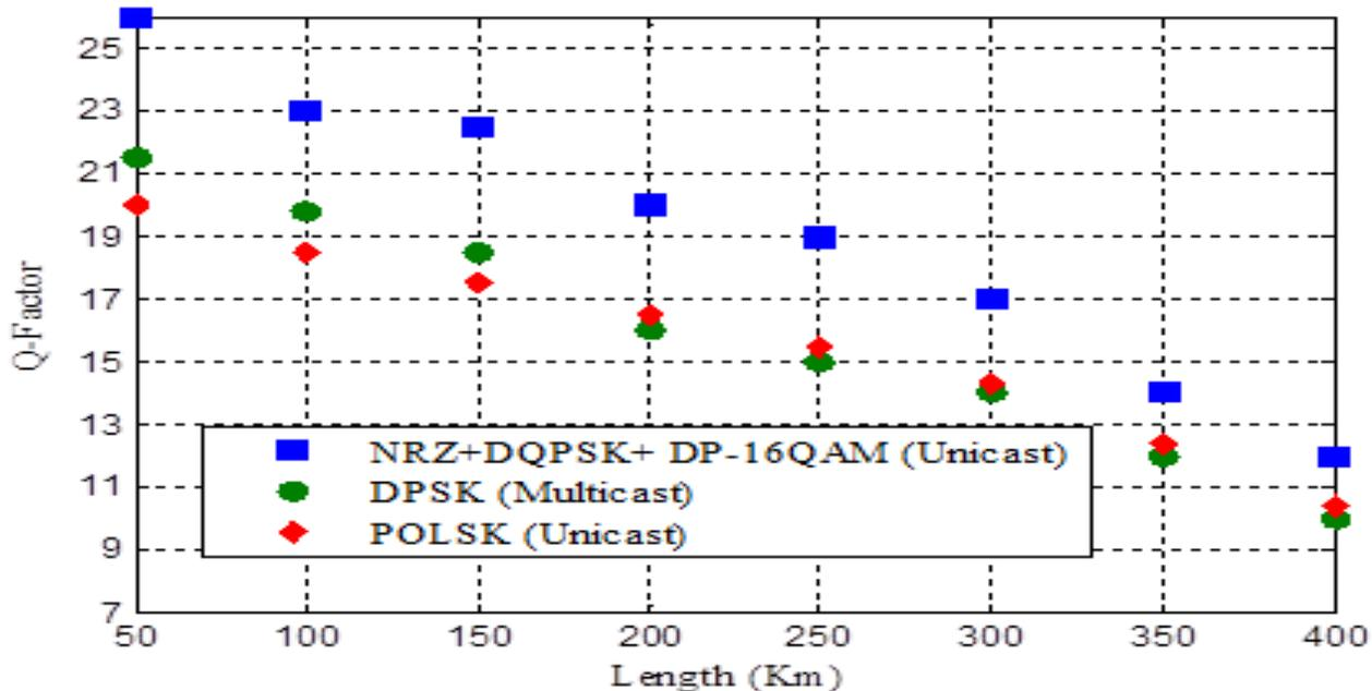
**Fig.4.** Performance Analysis of Quality-Factor w.r.t length for each channel using Unicast (NRZ+DQPSK+DP-16QAM and POLSK) and Multicast modulation (DPSK)
