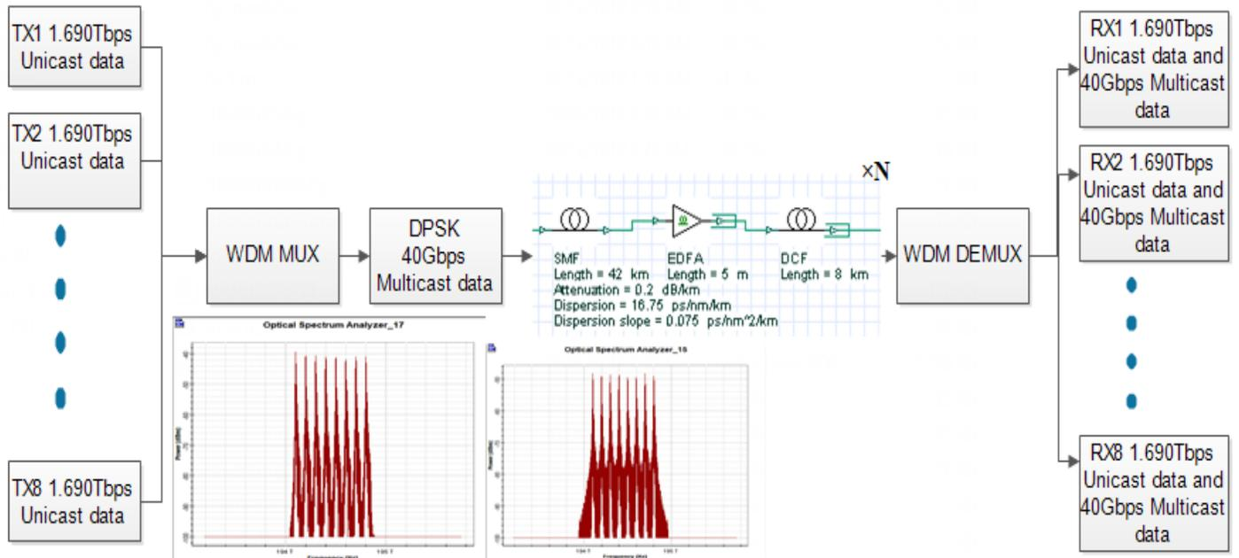
Fig.2. Schematic design of unicast signal overlay multicast signal
