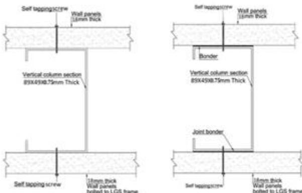
**Figure 2 Connection of ferrocement LGS composite**
