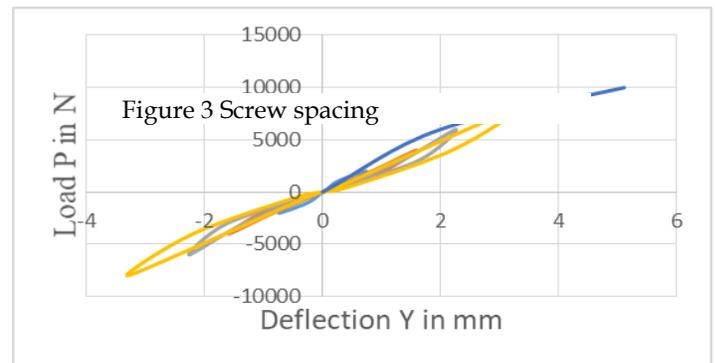
**Figure 4 Load vs Deflection of C-150**
