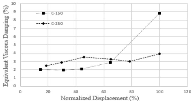
**Figure 9** Damping behaviour of flexure specimen
