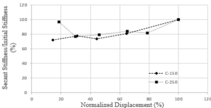
**Figure 10** Stiffness degradation of flexure specimen
