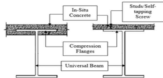
Figure 1 General used composite section
