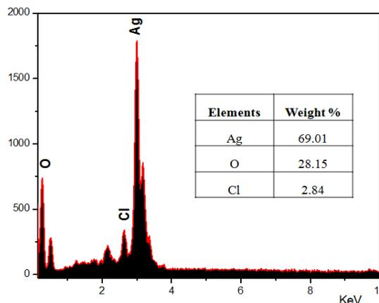
**Figure 8. EDX Spectrum of Ago Nanoparticles**
