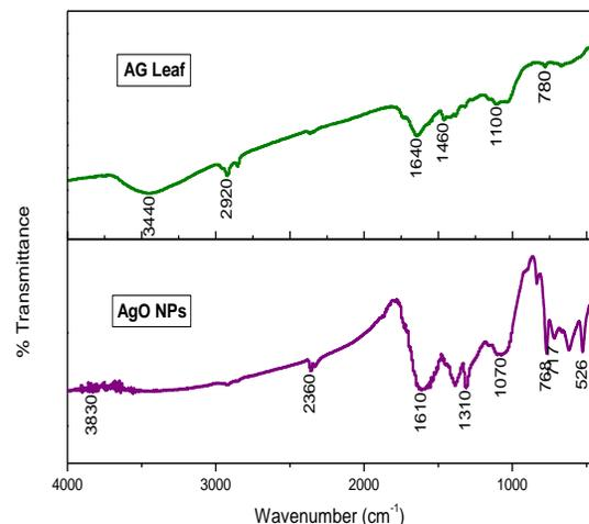
Figure 4. FTIR Spectra of AG leaves and AgO nanoparticles
