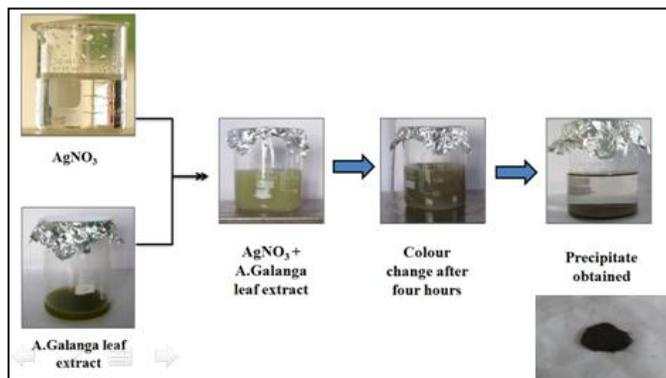
Figure 1: Reaction process using *A. galanga* and the obtained AgO Nanoparticles
