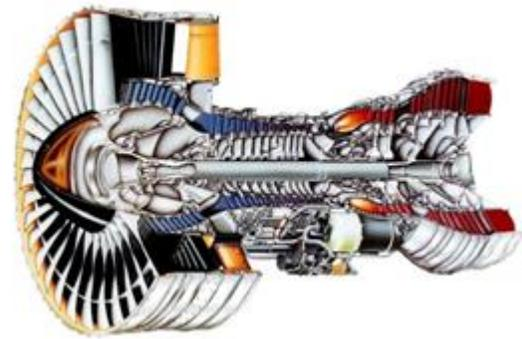
*Figure 1: A Typical Cross Section of PW4000-94 Inch Engine*
