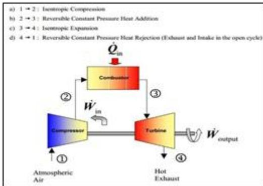
**Figure 2:** Closed-Cycle Gas Turbine
