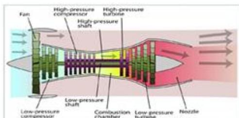
**Figure 3:** Components of a Turbofan engine
