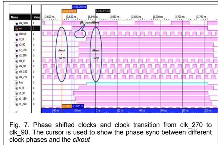
The system is designed and simulated using Xilinx 14.7 synthesis tool and tested its performance on SPARTAN 3E FPGA. The main components of the proposed design are VCO configured outside the FPGA, one on-chip PLL for frequency multiplication, one on-chip PLL with phase splitting feature, Clock selection circuitry and a Counter TDC.
