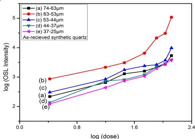
**Fig. 3.** OSL dose response curve for (a) 74-63 μm, (b) 63-53 μm, (c) 53-44 μm, (d) 44-37 μm and (e) 37-25 μm grain size samples of synthetic quartz.
