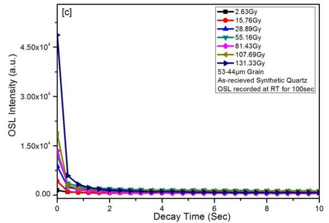
**Fig. 1(c).** OSL decay curve recorded at Room Temperature for 53-44  $\mu\text{m}$  grain size samples of synthetic quartz.
