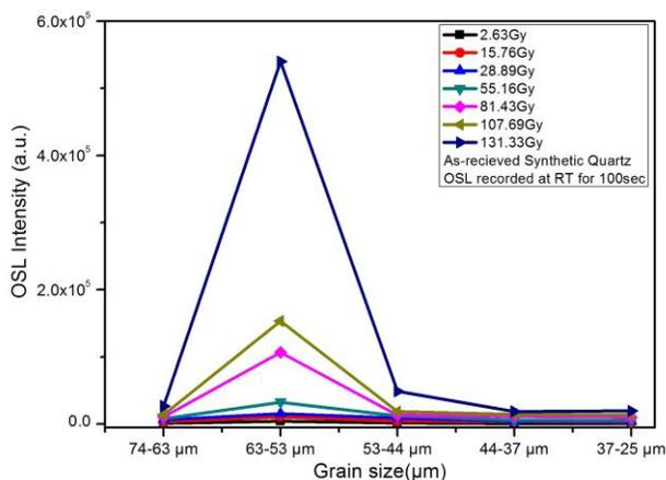
**Fig. 2** Comparative study of OSL intensity for different grain sizes at different beta radiation dose.
