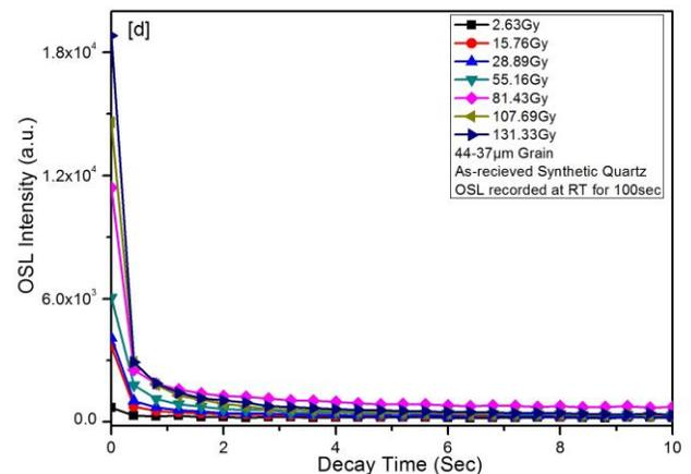
**Fig. 1(d).** OSL decay curve recorded at Room Temperature for 44-37  $\mu\text{m}$  grain size samples of synthetic quartz.
