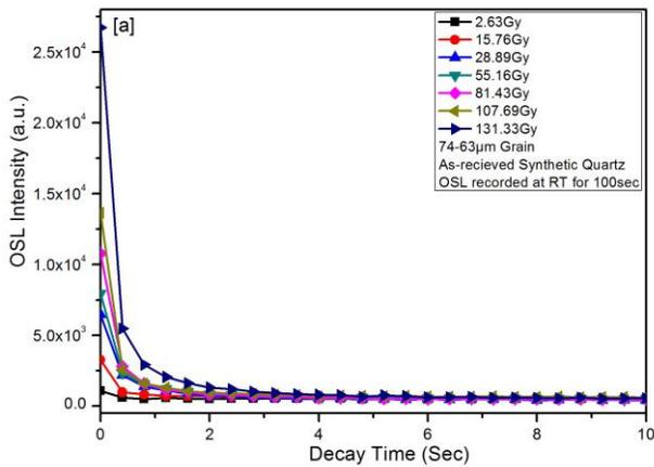
**Fig. 1(a).** OSL decay curve recorded at Room Temperature for 74-63  $\mu\text{m}$  grain size samples of synthetic quartz.
