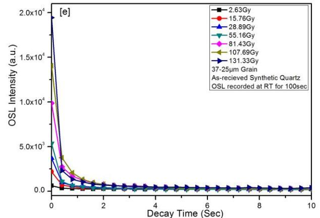
**Fig. 1(e).** OSL decay curve recorded at Room Temperature for 37-25  $\mu\text{m}$  grain size samples of synthetic quartz.
