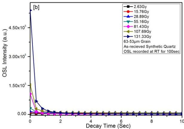
**Fig. 1(b).** OSL decay curve recorded at Room Temperature for 63-53  $\mu\text{m}$  grain size samples of synthetic quartz.
