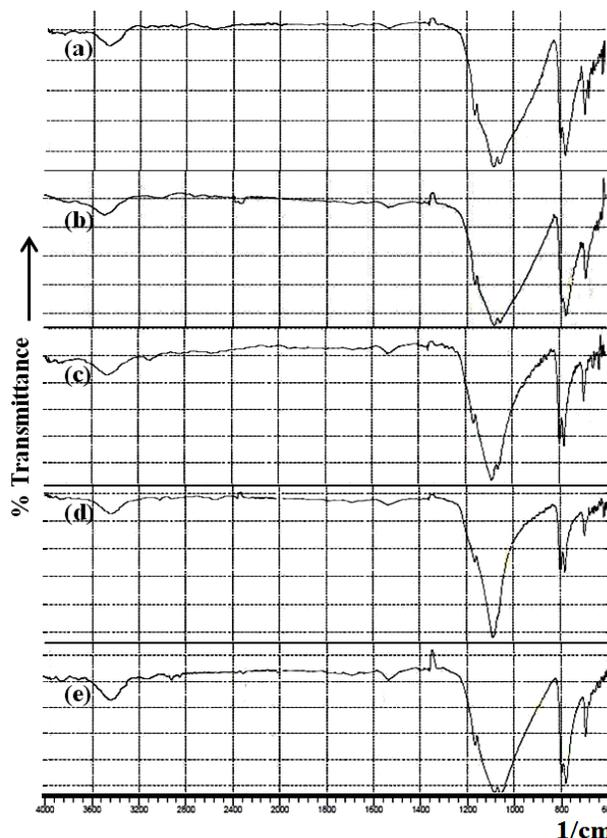
**Fig. 4.** FTIR spectrums for (a) 74-63 μm, (b) 63-53 μm, (c) 53-44 μm, (d) 44-37 μm and (e) 37-25 μm grain size samples of synthetic quartz.
