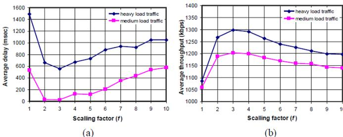
**Figure 4:** Average delay and average throughput as a function of scaling factor ( $f$ ), (a) average delay and (b) average throughput.
