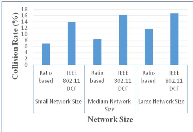
**Figure 6:** Collision rate as a function of network size for the Ratio Based and IEEE 802.11 DCF schemes.
