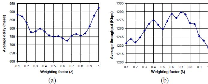
**Figure 3:** Average delay and average throughput as a function of weighting factor ( $\lambda$ ), (a) average delay and (b) average throughput.
