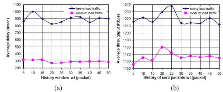
**Figure 5:** Average delay and average throughput as a function of history window ( $w_i$ ), (a) average delay and (b) average throughput.
