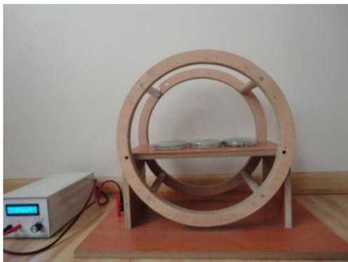
Fig. 1 electromagnetic field exposure arrangement
