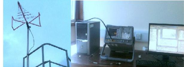
Fig 1. Measurement equipment employed in this study: Antenna, Spectrum Analyzer and Computer
