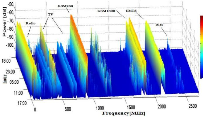
**Fig 3. Received power versus the frequency band (80MHz-2700MHz) for 24 hours**
