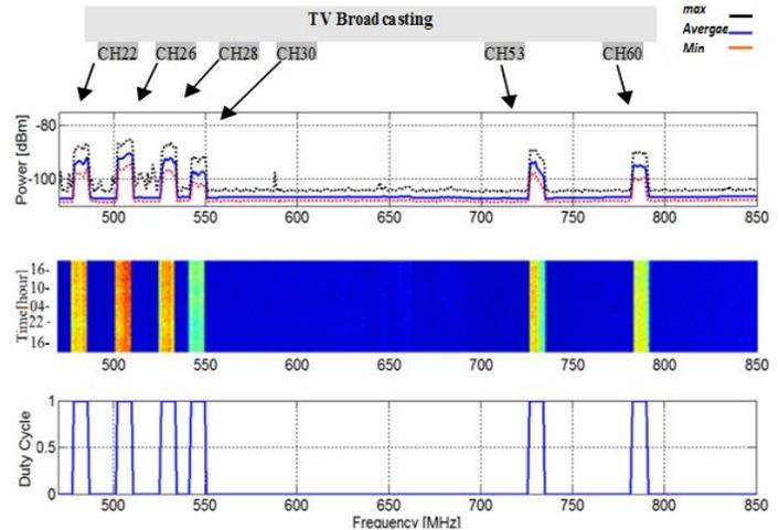
**Fig 5. Occupancy measurement from 470MHz to 850MHz**
