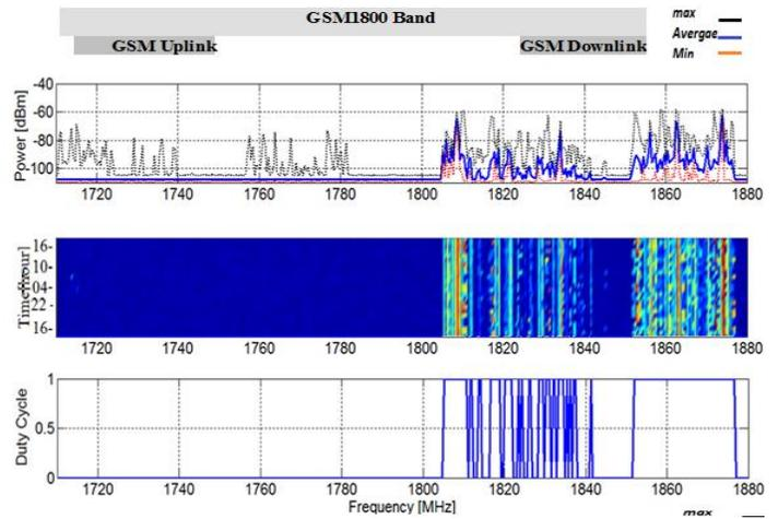
Fig 7. Occupancy measurement from 1710MHz to 1880MHz
