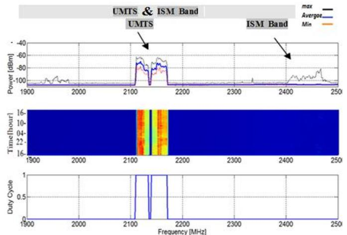
Fig 8. Occupancy measurement from 1900MHz to 2500MHz
