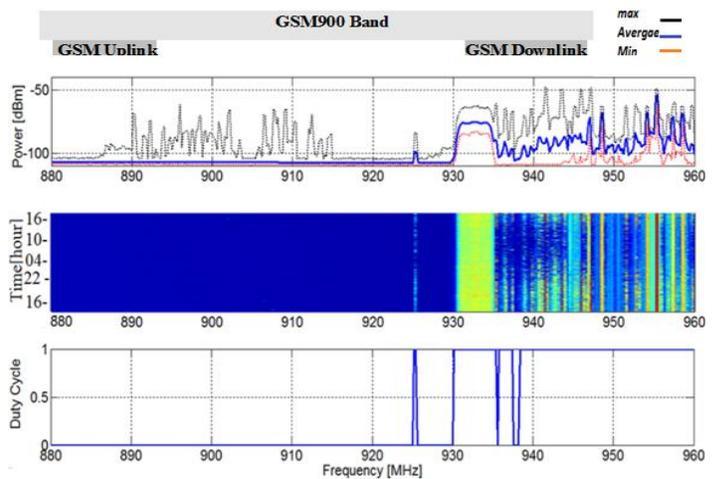
**Fig 6. Occupancy measurement from 880MHz to 960MHz**
