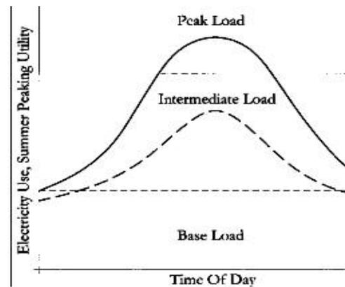
Fig 5: Typical Electric Load Curve [27]
