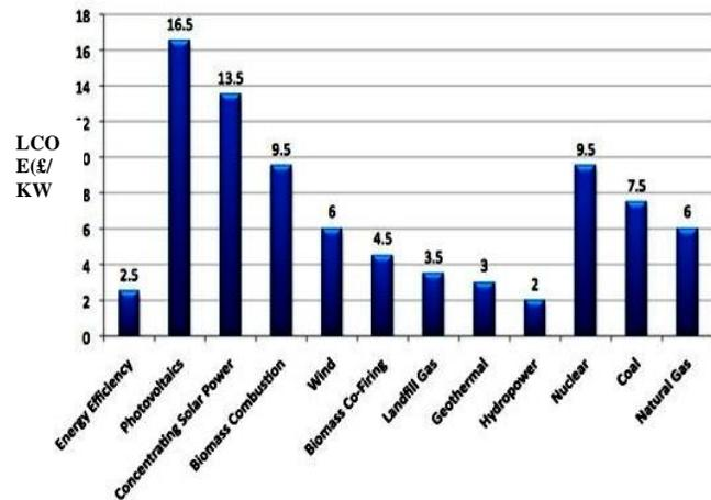
Fig 4: Levelised Cost of Energy for various power and energy efficiency option c/KWH [25]
