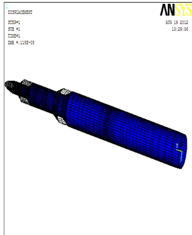
Fig 21: Deformation in the rocket outer shell when carbon-epoxy is considered (1).
