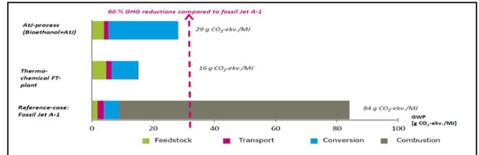
**Figure 1.** Comparison of Exhaust Emissions in Bioavtur Production and Avtur [26]
