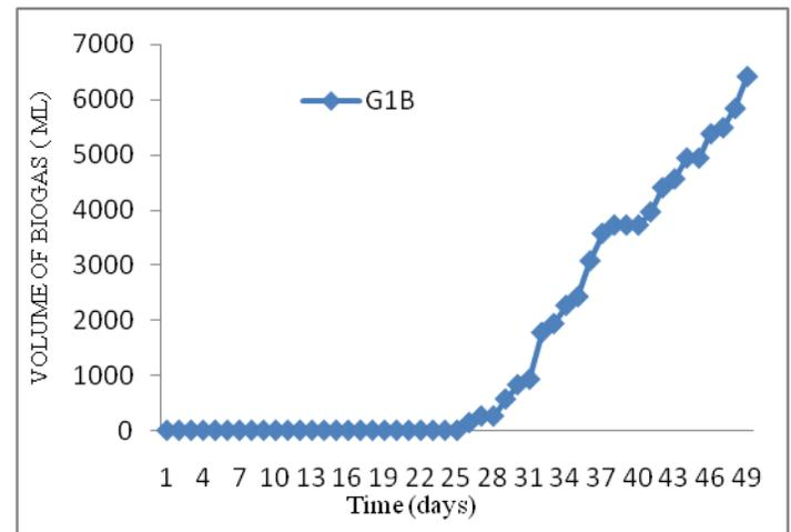
**Figure 3:** Cumulative Biogas Production for Digester G1B
