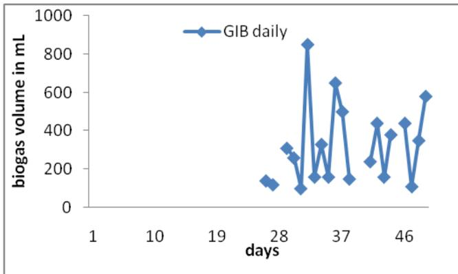
**Figure 4:** Daily biogas production from Digester GIB
