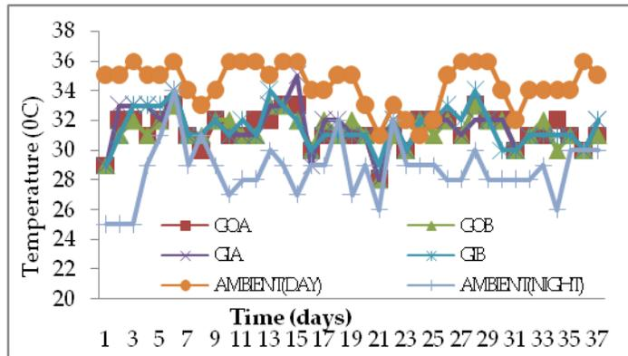
**Figure 1.** Digester's Internal and Ambient Temperatures
