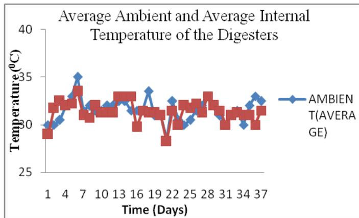
**Figure 2:** Digester's Average Internal and Ambient Temperatures
