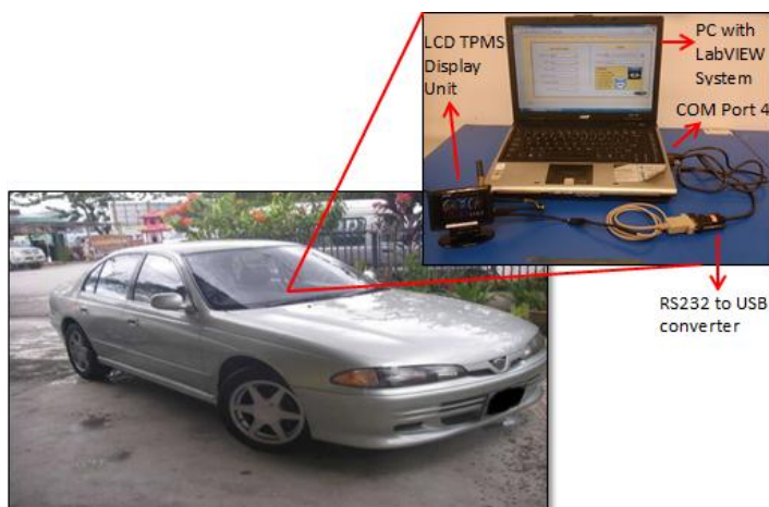
Fig 8. Tyre Pressure Deflation Test Setup on a Vehicle
