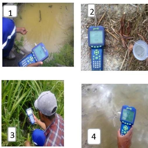
Fig.2. In situ measurement of physicochemical parameters
